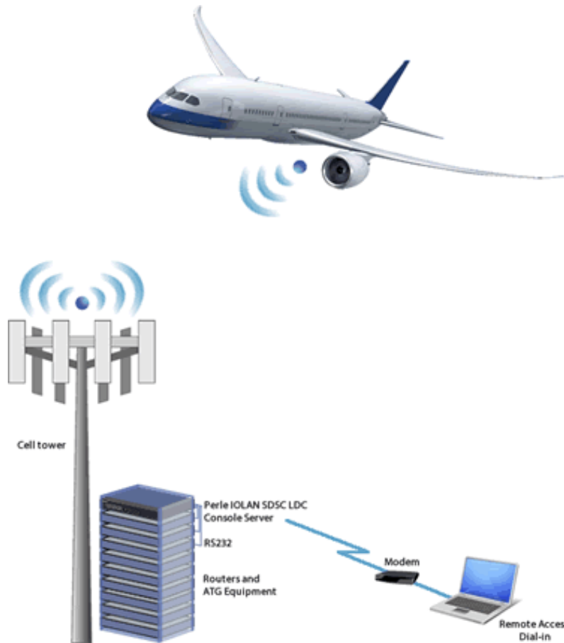
Operating an Air-to-Ground (ATG) 4G LTE In-flight Broadband Network
